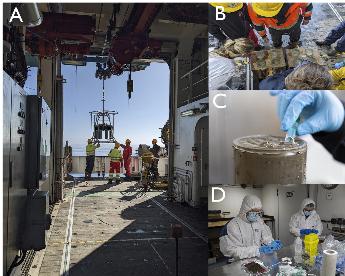
Figure 6.10. Photographic multipanel showing A) deployment of the megacorer, B) Assessment of the individual cores in the core rack, C) collection of eDNA samples from the top of the core using a cut-off syringe and D) collection of eDNA samples from core sections in the eDNA lab.
